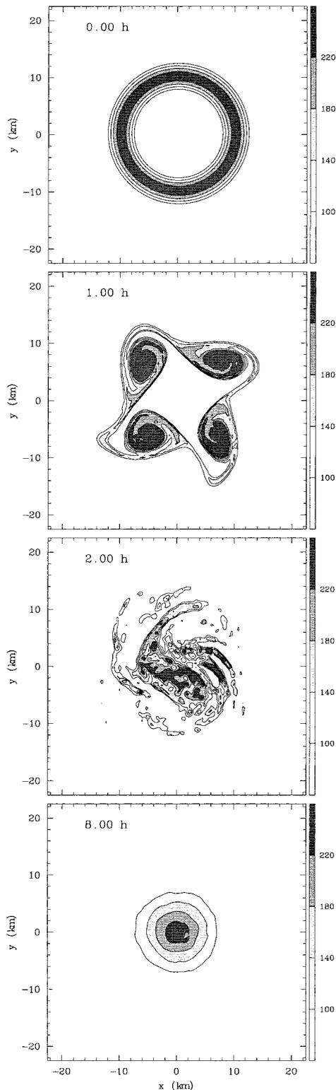
FIG. 10. Vorticity contour plots for expt. 7. The initial annulus rapidly relaxes to a monopole.
