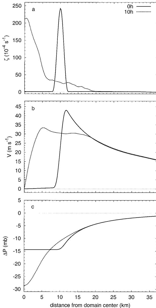
FIG. 7. Azimuthal mean (a) vorticity, (b) tangential velocity, and (c) pressure perturbation for expt. 2 at the selected times  $t = 0$  (solid) and 10 h (dashed). Averages were computed with respect to distance from the domain center. The pressure perturbation  $\Delta p$  is fixed at zero at  $r = 100$  km.
